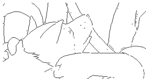
lines approximated by straight line and spline curve (total required dots for line-drawing: 509)
