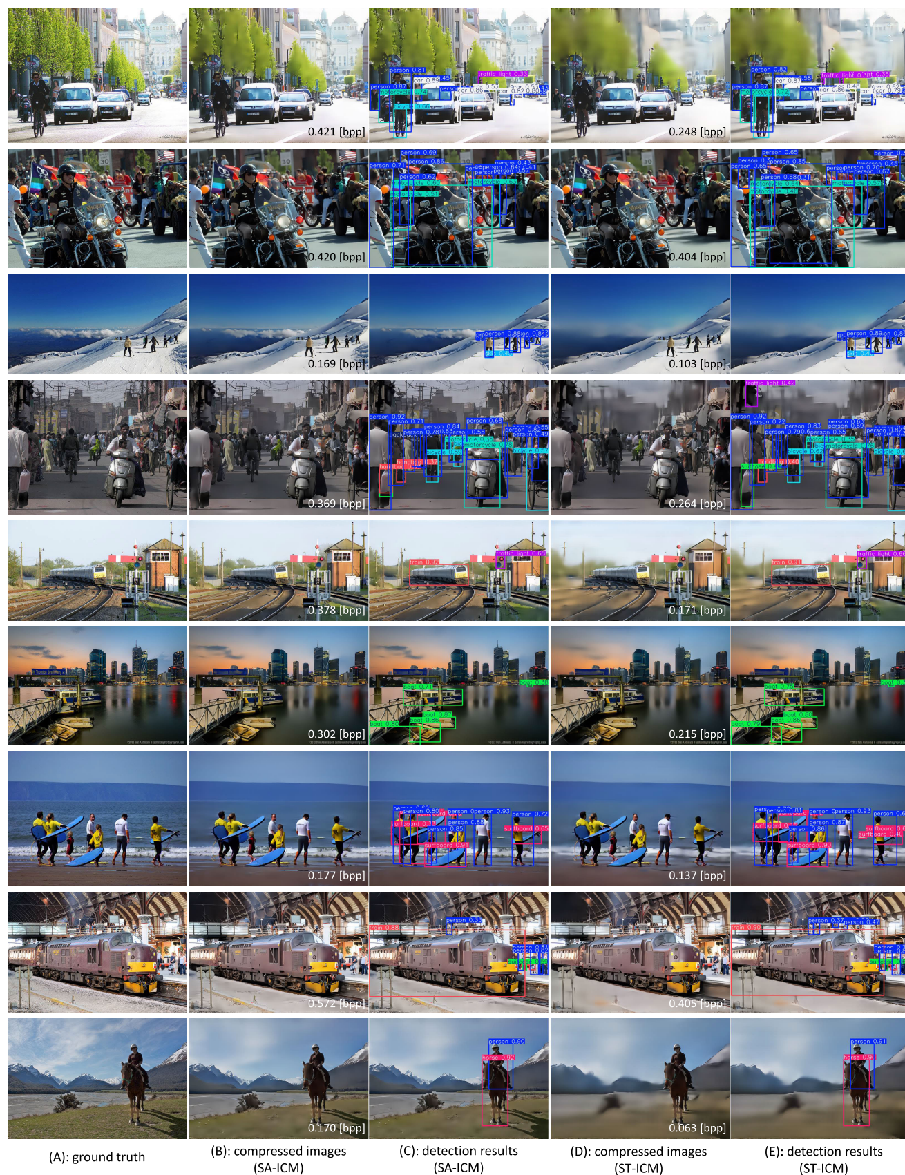
FIGURE 4. Example of decoded images and the results of detection by yolov5 on those images.
