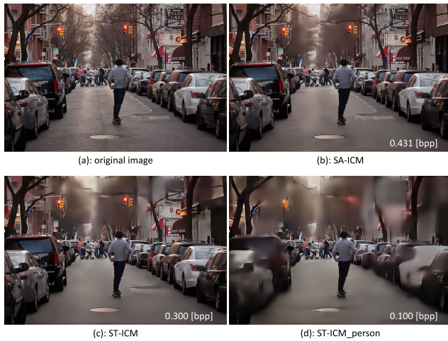
FIGURE 6. Examples of decoded images by each compression model. (a): original image, (b): decoded image with SA-ICM, (c): decoded image with ST-ICM, (d): decoded image with ST-ICM_person.
