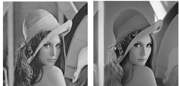
Figure 5: Original Lenna, 512*512 pels (left) and coded image (right) when using Canny edge detector with L_t=H_t=100 (SSIM=0.624, LPIPS=0.44, PSNR=15.05, Size=5.87KB).
