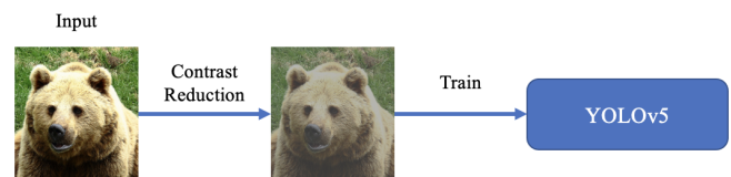
Fig. 1. Overview of contrast reduction and training process. Images that are processed by contrast reduction are used for validation as well. The image of the bear used in this figure is from the COCO2017 Val dataset, provided by Common Objects in Context (COCO) [11].
