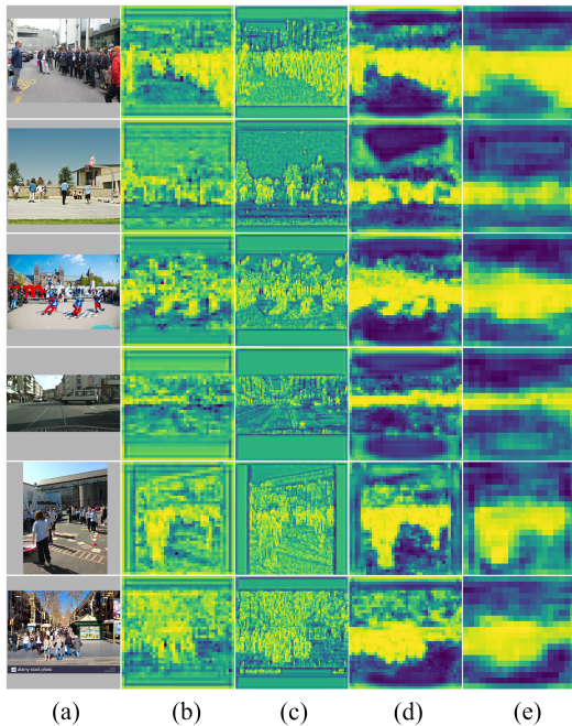
Fig. 3. Visualization of spatial attention within the Feature Transfer Block (FTB) on input images from the CrowdHuman Dataset. (a) is the input images in letter-box. The heatmaps (b), (c), (d), and (e) correspond to spatial attention visualization on f_{5 \rightarrow 4} , f_{4 \rightarrow 3} , f_{3 \rightarrow 4} , and f_{4 \rightarrow 5} , respectively.
