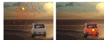
Fig. 1. Example of Deformable Convolution. Yellow dots show Convolution points and red dots show their receptive fields. The left image shows the case where the convolution point is in the background (sky), and the right image shows the case where the convolution point is in an object (car).
