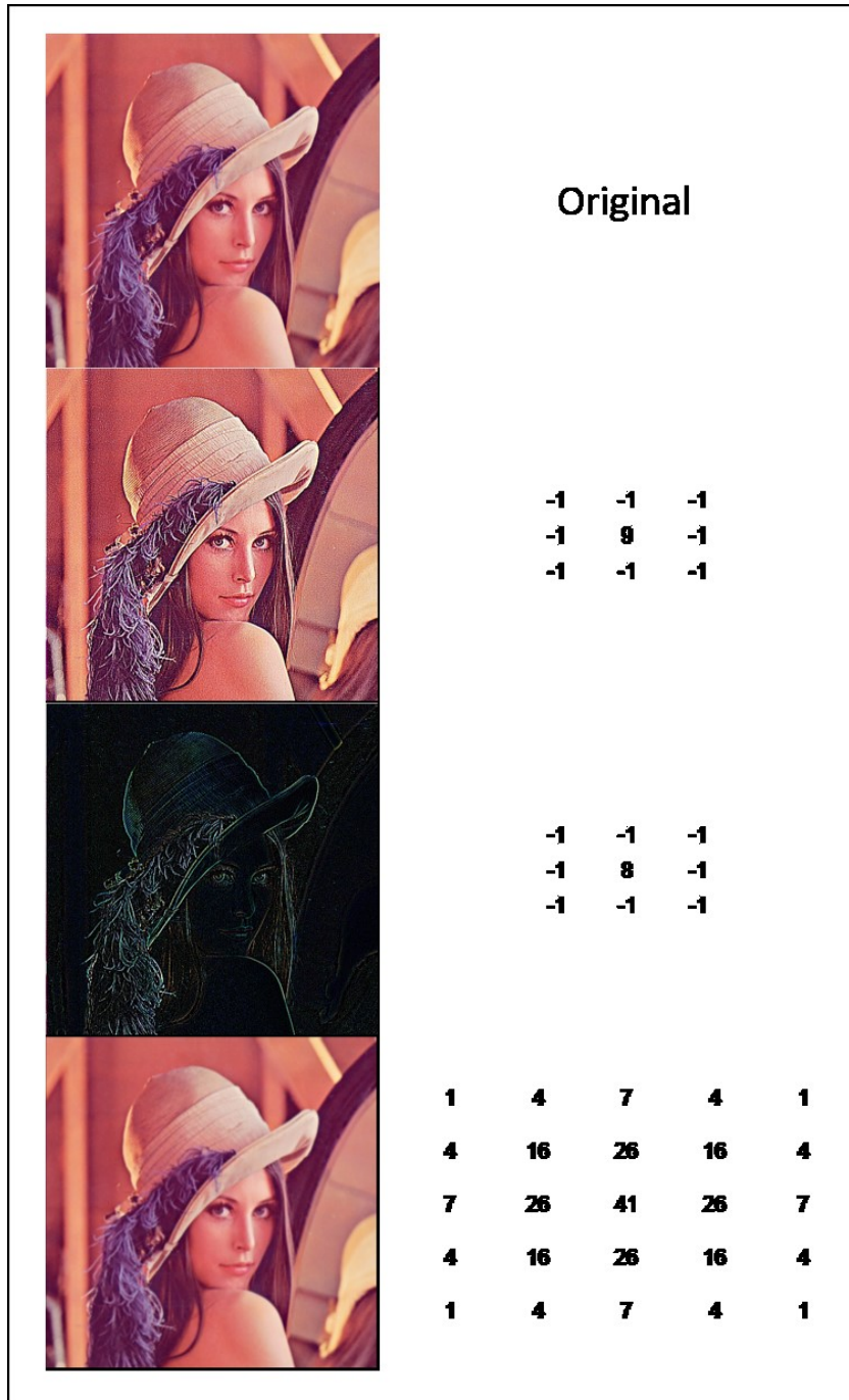
Figure 2.11 Convolution with Different Kernel
