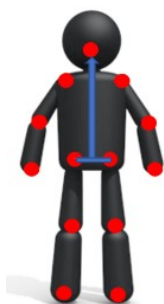
Fig. 3. Articulation points and vector diagram to be used in orientation estimation
