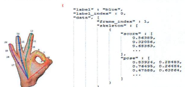
Fig. 2. (a) Hand Joints [2], and (b) Example x,y coordinates and its confidences
