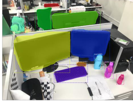
Figure 2.9: An example output of Mask R-CNN trained on COCO dataset
