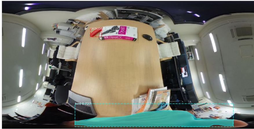
Figure 2.11: An example output of directly feeding EQR image into Mask R-CNN trained on COCO dataset, the performance is not good due to the non-uniform distortion (e.g., the book and TV are not detected)
