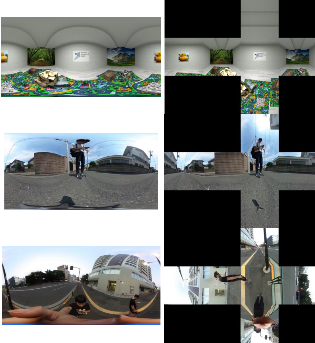
Figure 4.1: Example images taken from synthetic scene and real scene, left column shows raw EQR images, right column shows the counterpart preprocessed cubic images.
