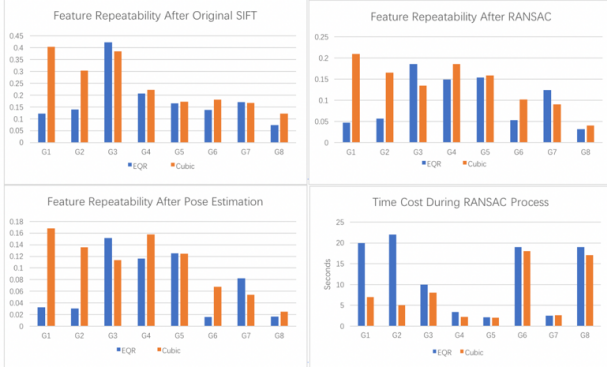
Figure.3. Comparison between EQR and Cubic image on performance of feature correspondences
