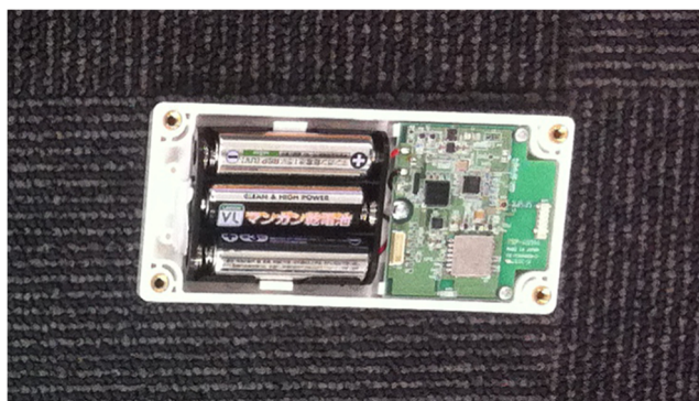
Fig. 2 Illustration of the Wi-Sun acceleration sensor, which can detect the acceleration values in the x-direction, y-direction and z-direction. The sensor also has the transmission module to broadcast the sensed data
