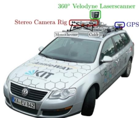
FIGURE 1.1: Different ways to collect input data in Visual Odometry (Image taken from KITTI website [9]).
