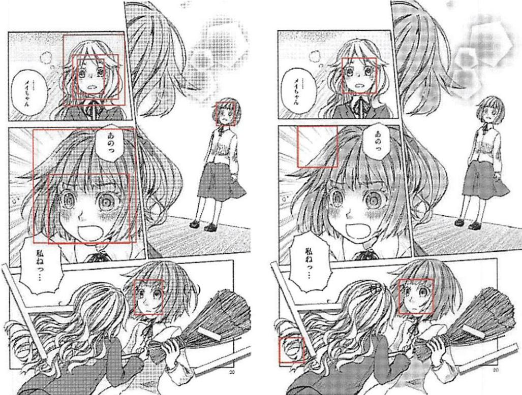
Fig. 6 (A) Result of face detection with DPM. (B) Result with HOG from same image. (Frames suggest detected area as character's face).
