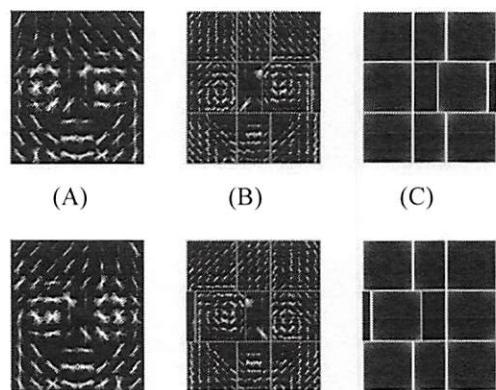
Fig. 5 Face detection model generated by DPM.
