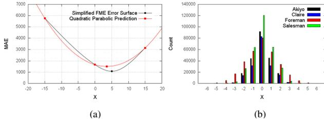
Figure 2. (a) An Example of the difference between real-world FME error surface and parabolic prediction model. (b) The matching counting by the distance between the best position of FFPS and that of PPBF.
